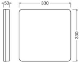
**Scheda tecnica Ledvance Bulkhead LED Surface Piatto Fonti luminose Piazza Bianca 16W 2660lm - 830-840 CCT | 300mm - IP20**
