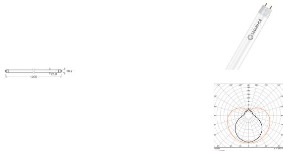
**Scheda tecnica Ledvance Tubo LED T8 EM Value Conventional (EM), Mains (AC) Ultra Output 20W 2160lm - 830 Luce Calda - | 120cm - Sostitutiva 36W**
